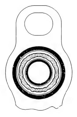
Seat of valve cone (1) and sealing surface of valve body (2) must not be dented, exhibit cavitation or show signs of uneven wear.
